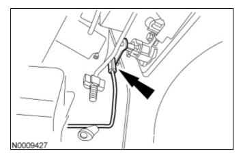
7. Disconnect the 2 wiring harness electrical connectors.
