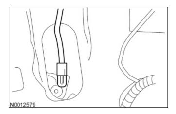
6. If equipped, disconnect the door lock cylinder actuating rod.
