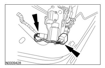
5. If equipped, connect the door lock cylinder actuating rod.
